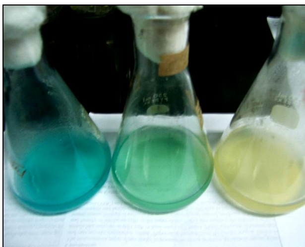
Fig 3. Daily decolorization of MG in nutrient broth culture of G. terrae from day 1 to day 2 to day 3 (left to right)
